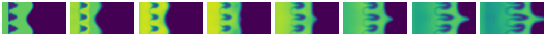
Figure 1: Snapshots of density in time increments of 0.1\mu\text{s} from left to right as an RMI forms.
