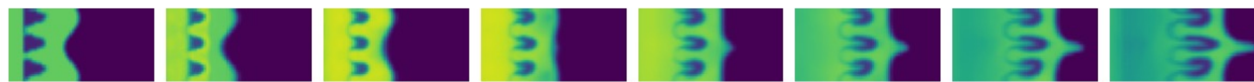
Snapshots of density in time increments of 0.1\mu\text{s} from left to right as an RMI forms.
