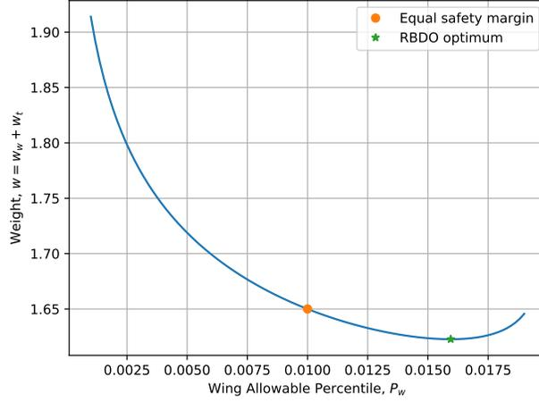
**Fig. 5 One dimensional plot along the constraint boundary shows the new RBDO optimum and the location of the previous UAV design, where the wing and tail used the A-basis allowable from the Hanson-Koopmans method.**
