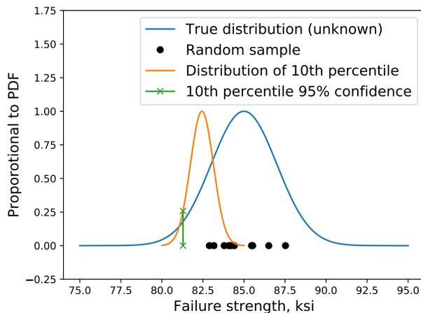
**Fig. 1 Illustration of approximating the 10<sup>th</sup> percentile with 95% confidence from a random sample which comes from an unknown distribution.**
