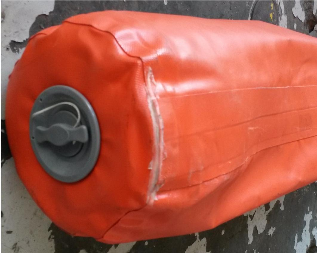
**Figure 6.2:** Inflatable cylinder valve on the end cap and seam running down the length of the cylinder
