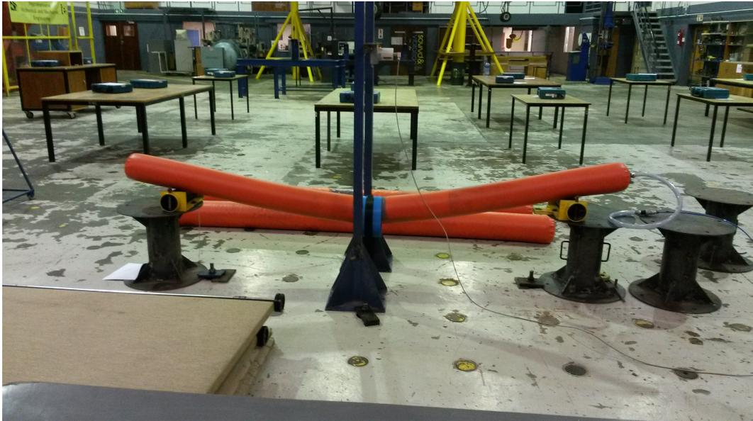
**Figure 6.3:** 150 mm inflatable cylinder bending in the test setup
