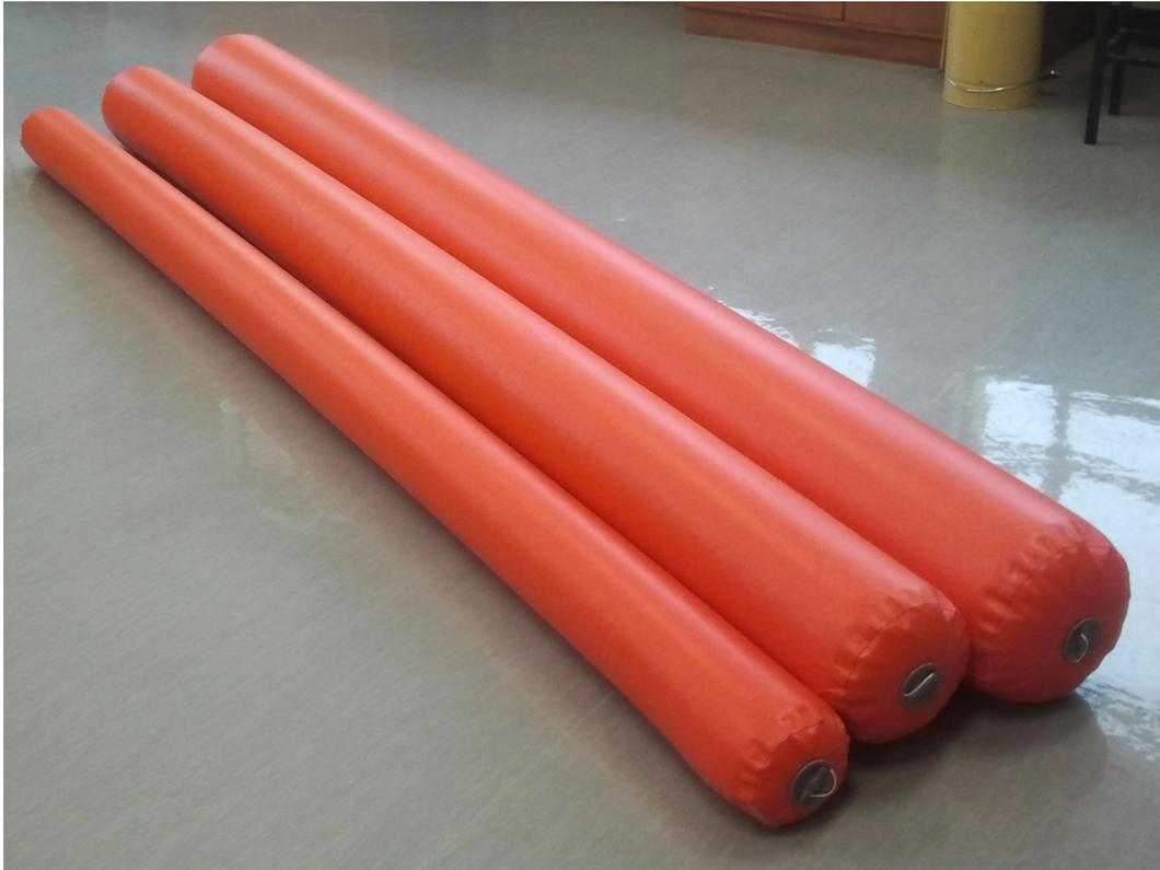
**Figure 6.1:** Three PVC-coated polyester cylinders with diameters of 150 mm, 200 mm, 250 mm
