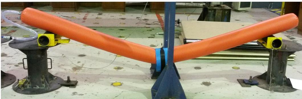
**Figure 6.8:** 150 mm diameter inflatable cylinder at the buckling load in the three point bending test configuration
