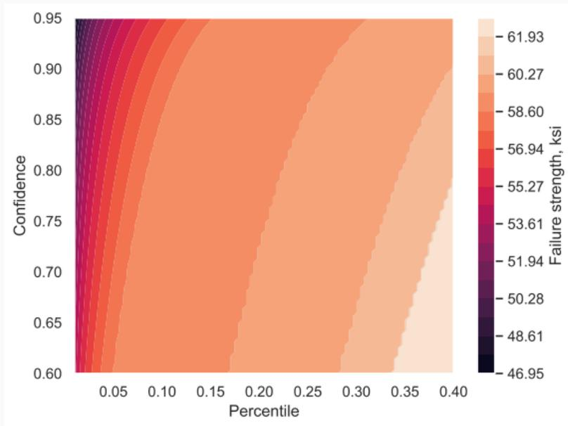
**Figure 4:** With just 18 samples, the Hanson-Koopmans tolerance interval can be calculated for any percentile and confidence.
