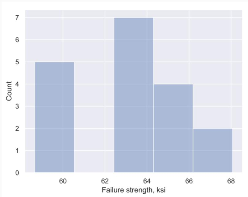
Figure 1: Histogram of 18 tension tests on composite material.
