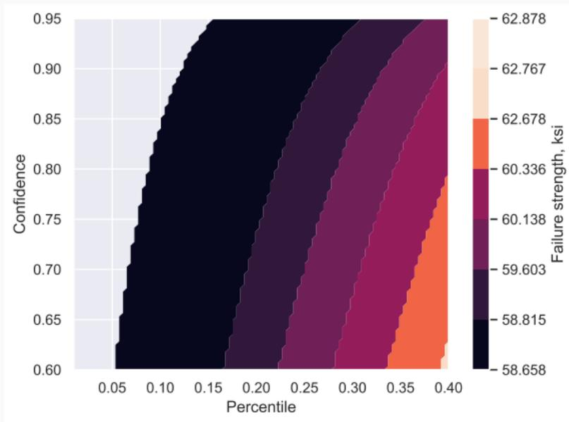
**Figure 3:** With just 18 samples, the non-parametric tolerance interval is limited to certain percentile confidence levels.
