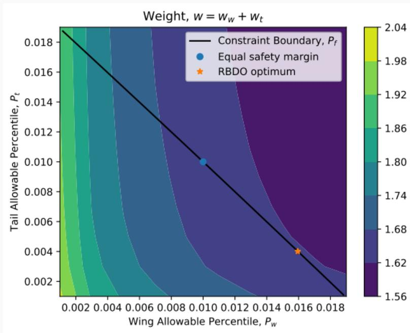
**Figure 7:** Contour plot of the objective function when using the Hanson-Koopmans method.
